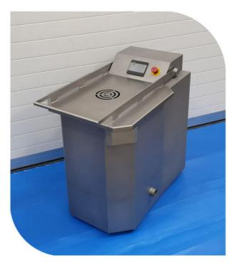
Integrated safety system prevents access to the spinning chamber whilst the spinner is operational to reduce risk to the operators.
