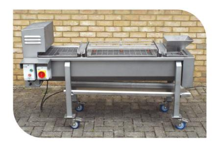
The WB Sliver Remover now comes with the option of a single point adjustment system to simplify the transition between sliver thicknesses.
